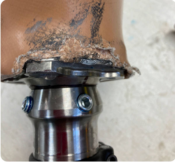
Example of delamination at the distal end.
