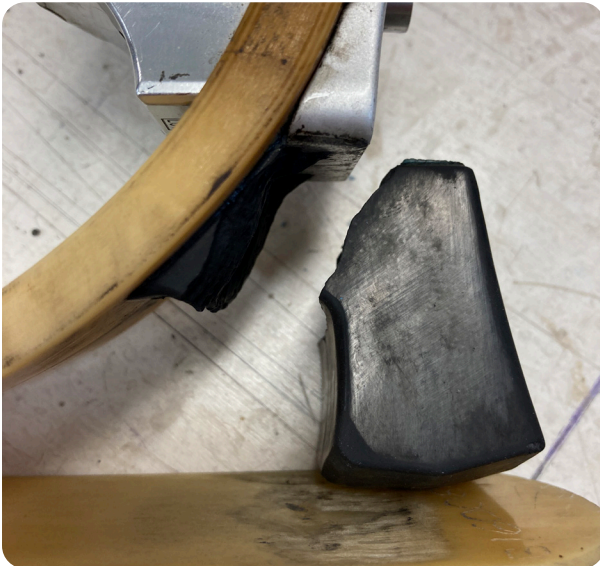
Example of foot heel rubber failure.
