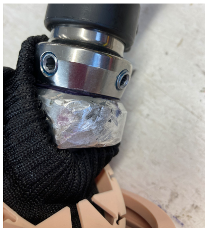
Example of delamination at the distal end.
