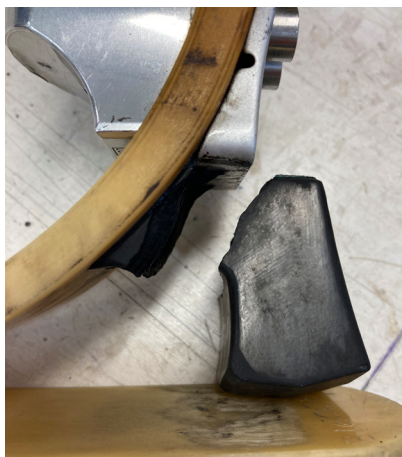
Example of foot heel rubber failure.
