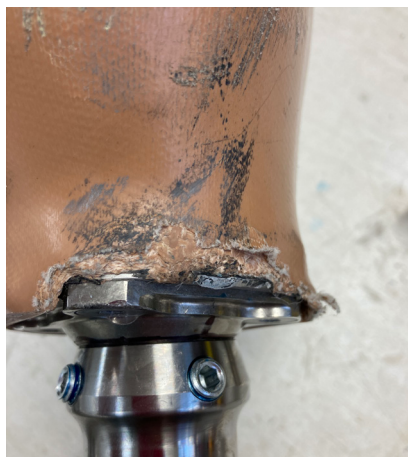
Example of delamination at the distal end.
